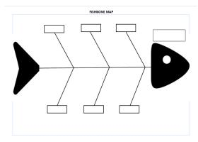
Firstly, the **fishbone diagram** can help you consider cause and effect with opportunity to consider large numbers of causes. The problem to be considered is placed in the box by the fish head and then the fish bones are used to describe and explain all the different causes that need to be considered.
